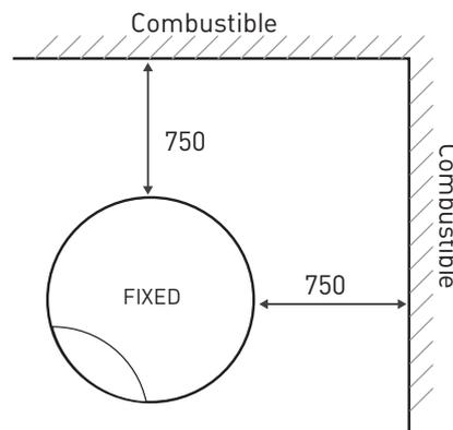
Clearances may be reduced with the application of heat shielding to walls in accordance to the Australian Building Code.
