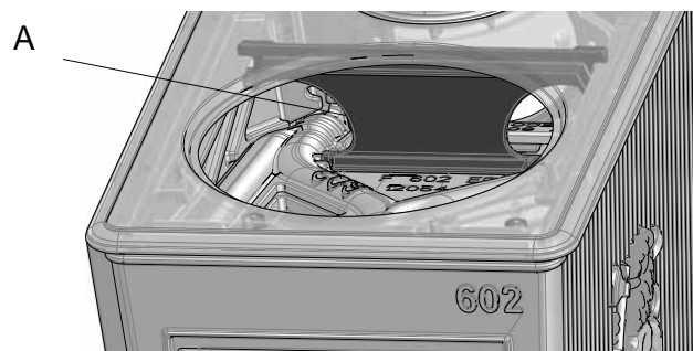
Fig. 28 Replacing the exhaust reflector
